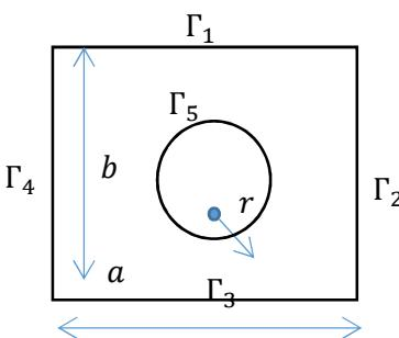
$$\frac{\partial u}{\partial n} = \begin{cases} 1 & (x, y) \in \Gamma_1 \\ 0 & (x, y) \in \Gamma_2 \cup \Gamma_4 \cup \Gamma_5 \end{cases}; \quad u|_{\Gamma_3} = 0$$
