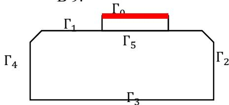
$$\frac{\partial u}{\partial n} = \begin{cases} 1 & (x, y) \in \Gamma_0 \\ 0 & (x, y) \in \Gamma_1 / \Gamma_5 \cup \Gamma_2 \cup \Gamma_4 \end{cases}; \quad u|_{\Gamma_3} = 0$$
