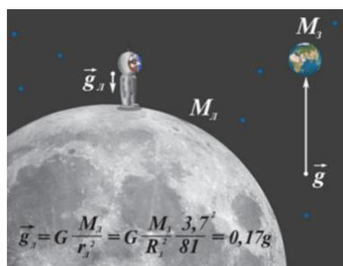
$$g_L = G \frac{M_L}{R_L^2} = G \frac{M_3 \cdot 3,7^2}{T_3^2 \cdot 81} = 0,17g = 1,66 \text{ м/с}^2$$
