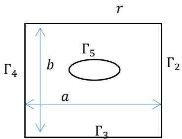
$$\frac{\partial u}{\partial n} = \begin{cases} 1 & (x, y) \in \Gamma_1 \\ 0 & (x, y) \in \Gamma_2 \cup \Gamma_4 \cup \Gamma_5 \end{cases}; \quad u|_{\Gamma_3} = 0$$
