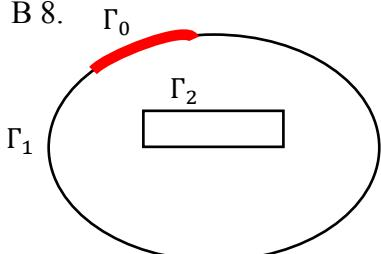
$$\frac{\partial u}{\partial n} = \begin{cases} 1 & (x, y) \in \Gamma_0 \\ 0 & (x, y) \in \Gamma_1 / \Gamma_0 \cup \Gamma_2 \end{cases}$$
