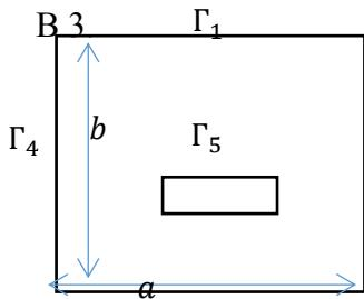
$$\frac{\partial u}{\partial n} = \begin{cases} 1 & (x, y) \in \Gamma_4 \\ 0 & (x, y) \in \Gamma_1 \cup \Gamma_2 \cup \Gamma_5 \end{cases}; \quad u|_{\Gamma_3} = 0$$
