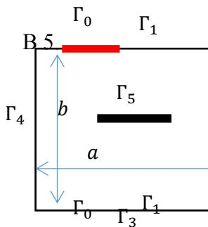
$$\frac{\partial u}{\partial n} = \begin{cases} 1 & (x, y) \in \Gamma_0 \\ 0 & (x, y) \in \Gamma_1/\Gamma_0 \cup \Gamma_2 \cup \Gamma_4 \end{cases}; \quad u|_{\Gamma_3} = 0$$
