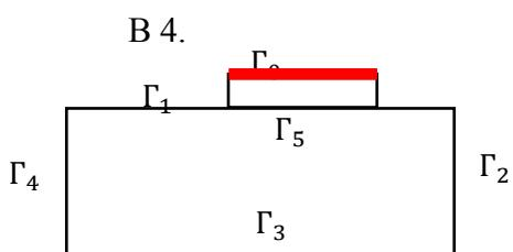
$$\frac{\partial u}{\partial n} = \begin{cases} 1 & (x, y) \in \Gamma_0 \\ 0 & (x, y) \in \Gamma_1/\Gamma_5 \cup \Gamma_2 \cup \Gamma_4 \end{cases}; \quad u|_{\Gamma_3} = 0$$
