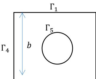
$$\frac{\partial u}{\partial n} = \begin{cases} 1 & (x, y) \in \Gamma_1 \\ 0 & (x, y) \in \Gamma_2 \cup \Gamma_4 \cup \Gamma_5 \end{cases}; \quad u|_{\Gamma_3} = 0$$
